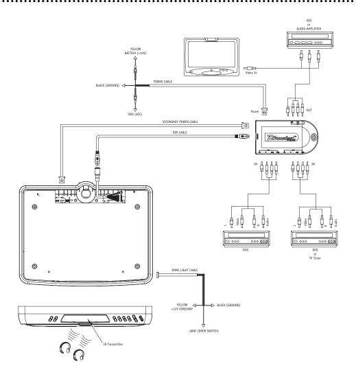
**NOTE:** The Second Power cable must be connected or the unit will not operate and will cause damage to the unit.
